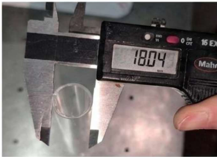
Physical measurement with a vernier caliper ( \phi 18 pipe)
